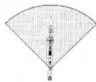
Deck/Sail array (aft) sonar baffles (dead zone)
