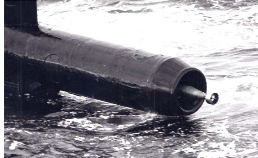
Project 667BDR SSBN towed array with drogue
