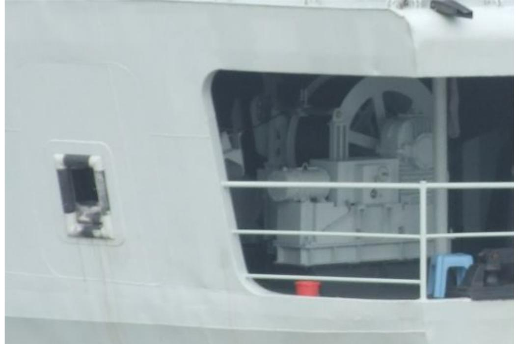
Type 053H2G (JAINGWEI I) frigates 540 and 542 both have modifications to their sterns for a towed device of some kind. Internet photos have linked *Huainan* (Hull 540) as being equipped with a towed array and the deployment port is similar in configuration and location to that on the Type 054A. Unfortunately, the presence of the handling system and reel does not clarify which option is more likely as only a single cable-wrapped reel can be seen.
