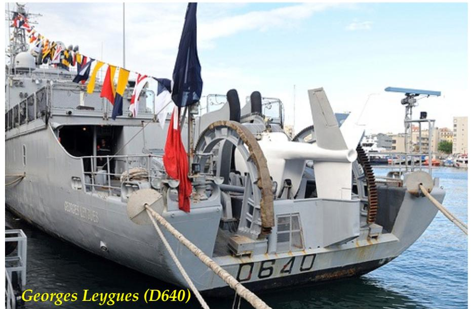
The French DUBV-43 VDS uses a large towed body and the beefy MSR 2D handling system. Together, the VDS and the handling system weigh approximately 100.8 metric tons, or 111.1 short tons. The towed body's large size is driven by the sonar array's frequency, which is centered on 5.0 kHz and is classified as a medium frequency sonar.
