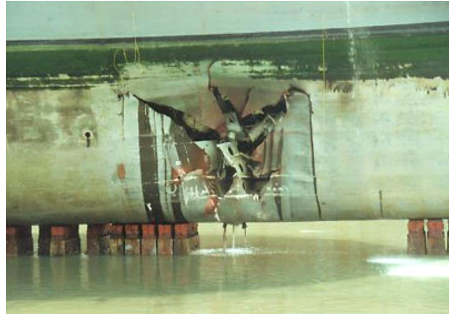
*USS Tripoli contact mine damage*
