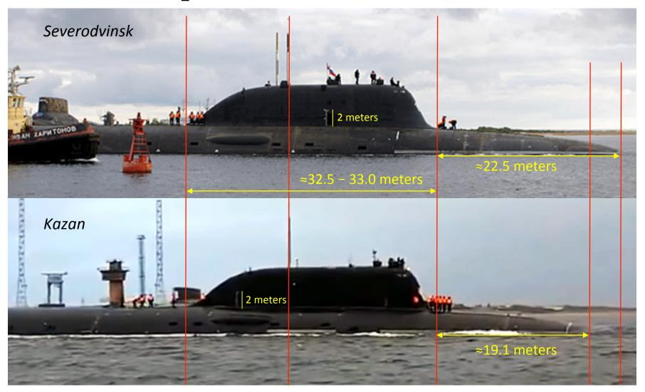
A comparison of the two boats from a nearly identical aspect, with the sail draft markings in view, shows the bow of *Kazan* is about 3.5 meters shorter than *Severodvinsk*, above the waterline. The sail length on both submarines is essentially identical at 32.5 - 33.0 meters.
