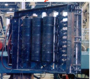
Integrated passive conformal and flank arrays
