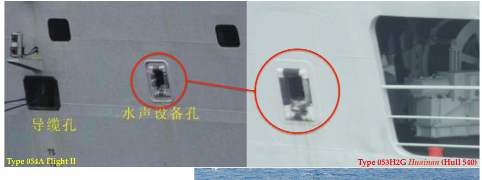
The towed array deployment port on Type 054A Flight II ships is virtually identical with the one found on the Type 053H2G JAINGWEI I frigates *Huainan* (Hull 540) and *Tongling* (Hull 542). This strengthens the argument that the ports share the same function.
