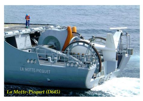
The French DUBV-43 VDS uses a large towed body and the beefy MSR 2D handling system. Together, the VDS and the handling system weigh approximately 100.8 metric tons, or 111.1 short tons. The towed body's large size is driven by the sonar array's frequency, which is centered on 5.0 kHz and is classified as a medium frequency sonar.
