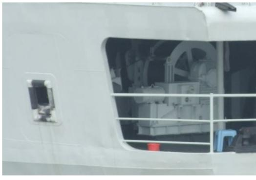
Type 053H2G (JAINGWEI I) frigates 540 and 542 both have modifications to their sterns for a towed device of some kind. Internet photos have linked *Huainan* (Hull 540) as being equipped with a towed array and the deployment port is similar in configuration and location to that on the Type 054A. Unfortunately, the presence of the handling system and reel does not clarify which option is more likely as only a single cable-wrapped reel can be seen.
