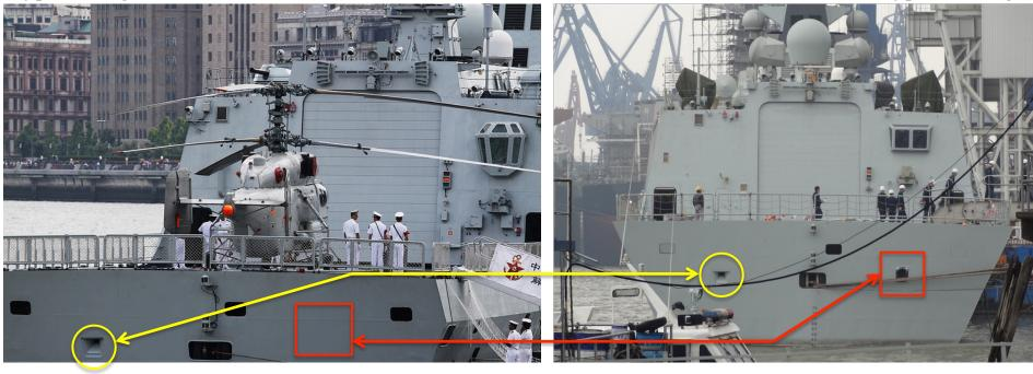
There is an intriguing difference between the Type 054 and the Type 054A frigates. The port opening is present on both classes, but the Type 054 *does not* have a starboard opening. Tactically, it makes more sense that both classes be fitted with a torpedo decoy system rather than a towed array.
