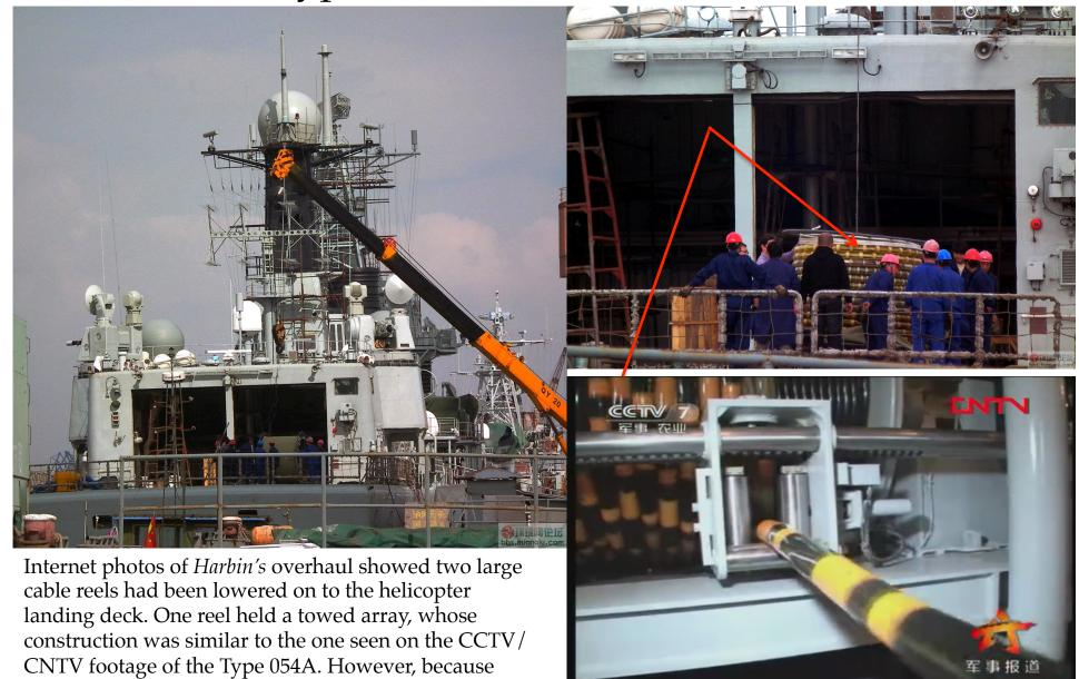
only one stern opening was seen, the Type 052 destroyers do not have a towed torpedo decoy.
