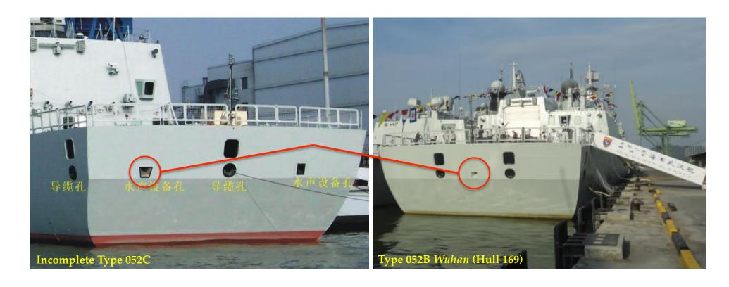
The configuration of the Type 054A Flight II frigates can also serve as an indicator for other PLAN ships. Case in point, all Type 052C destroyers have a very similar stern arrangement with a towed decoy opening to port and a towed array opening to starboard. The Type 052B destroyers only have a towed decoy opening at the center of the transom. From this it can be concluded that the Type 052B DDGs *will not* be fitted with a towed array, while the Type 052C will have one.
